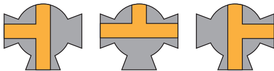
Flow Plan 1: 3 Way, 3 Port, 180° turn, 3 Positions
